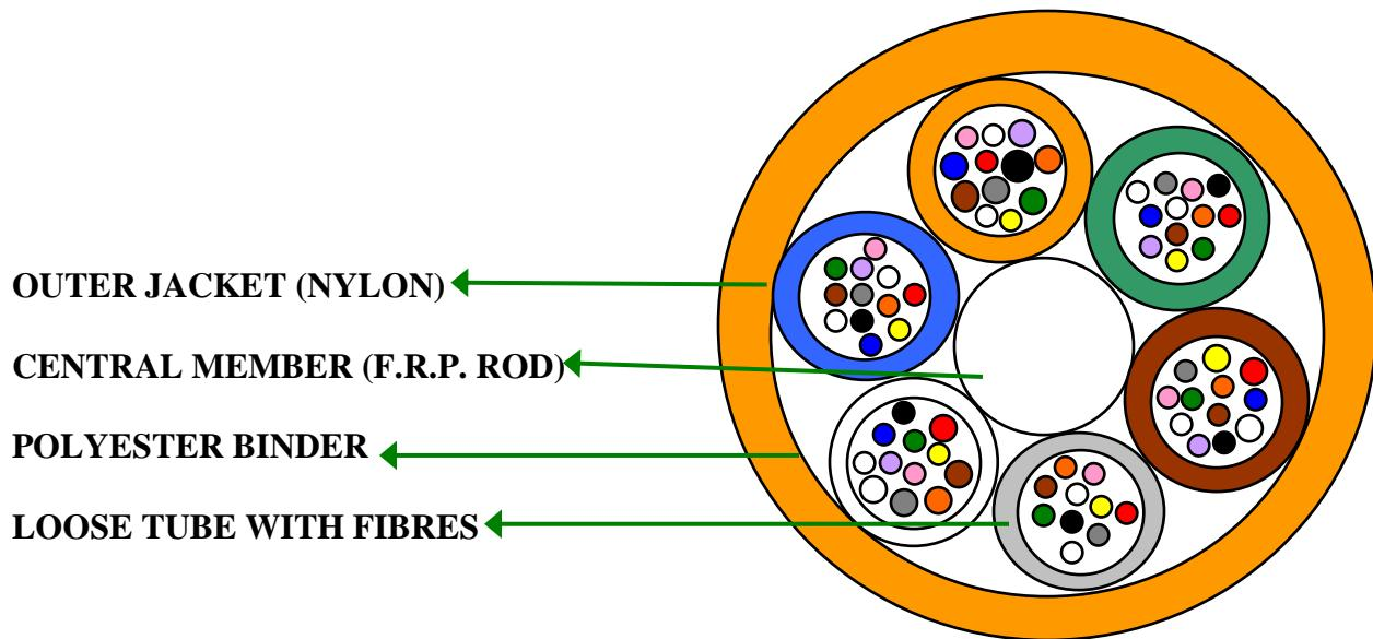
**3.9.3 Strength Member :** Solid non-metallic strength member (FRP) shall be provided in the center of the cable core. The strength member (as per Annexure-II) in the cable shall be for strength and flexibility to the cable and shall have anti buckling properties.
