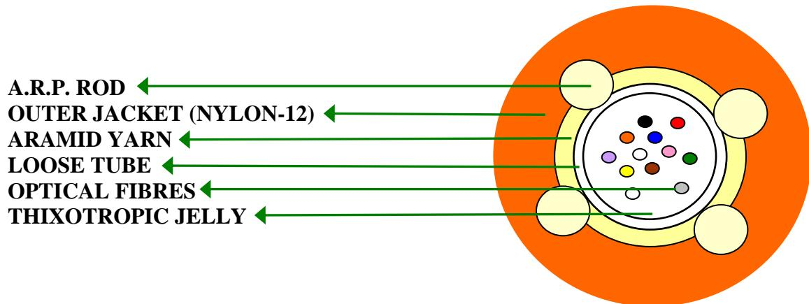
**3.8.4 Filling compound :** The filling compound used in the loose tube shall be compatible to fibre, secondary protection of fibre etc. The drip point shall not be lower than +70 degree C. The fibre movement shall not be constrained by stickiness and shall be easily removable for splicing. The filling jelly compound shall be as per the GR no. GR/ORM-01/03. MAR 04 and subsequent amendments, if any.
