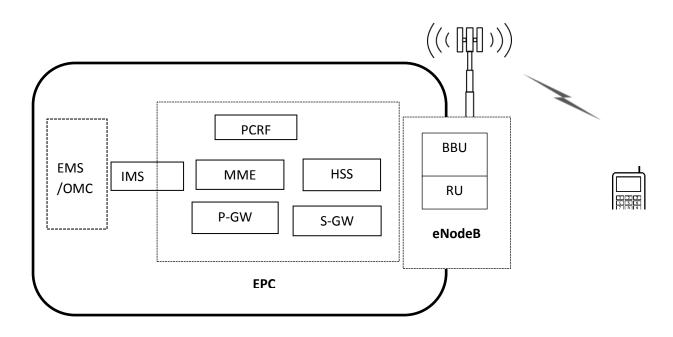
Fig 1: Compact LTE Mobile System
