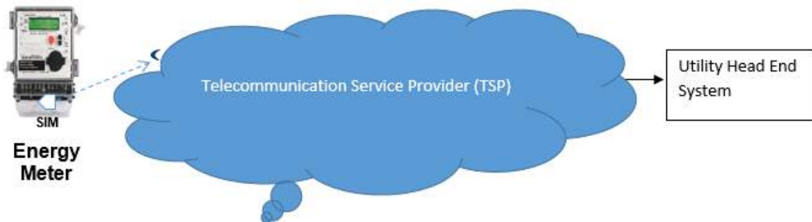
FIGURE 9 - IMPLEMENTATION SOLUTION TYPE 2: FOR METERING OF CONSUMERS AT SCATTERED LOCATIONS
