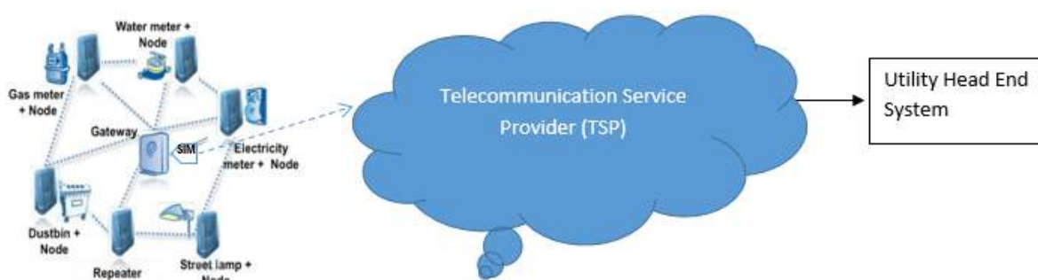
FIGURE 7 - IMPLEMENTATION SOLUTION TYPE 1: LOCAL MESH WITH REMOTE APPLICATION SERVER
