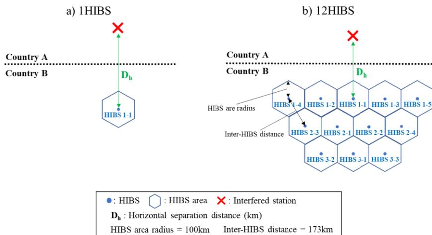
**A3.5.1.4.2.2 Calculation method of horizontal separation distance**
