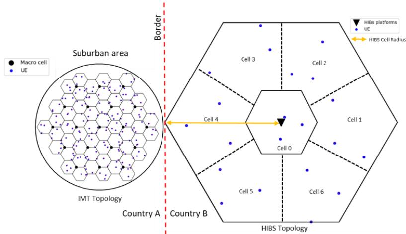
The simulation for co-channel sharing analysis was done considering both HIBS and IMT central frequency at 2 680 MHz, as shown in Figure A4.1.2.4.
