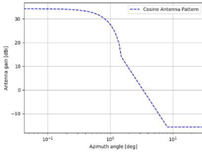
(a) Azimuth antenna pattern
