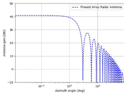
**(a) Azimuth antenna pattern**
