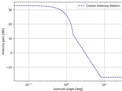
(a) Azimuth antenna pattern
