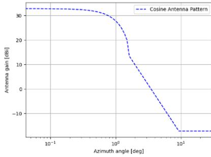
(a) Azimuth antenna pattern
