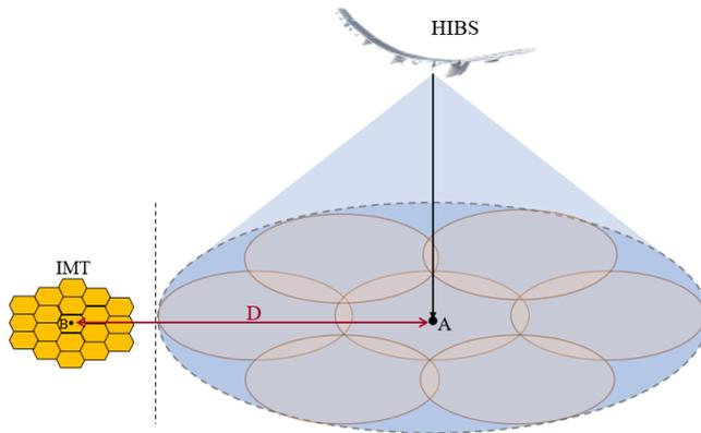
*Step 1.2: Determine the deployment of HIBS and the ground component of IMT system.*
