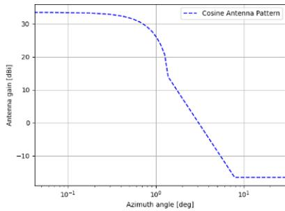
(a) Azimuth antenna pattern
