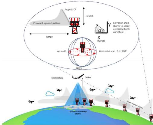
**Radar A: antenna height = 8 m, receiver noise figure = 4 dB, horizontal scan: -180° to 180°**
