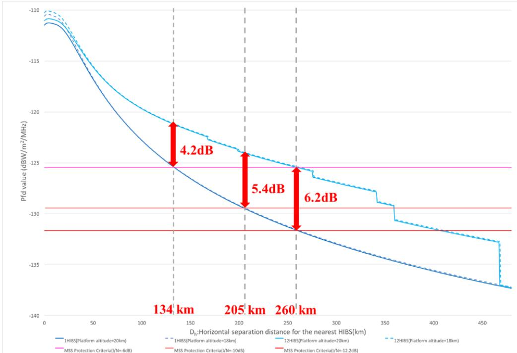
Based on the calculation result, the horizontal separation distance  $D_h$  to satisfy pfd values of non-GSO System R in Table A3.5.1.1 were 134 km ( $I/N=-6$  dB), 205 km ( $I/N=-10$  dB) and 260 km ( $I/N=-12.2$  dB) in the single HIBS deployment scenario with both 18 km and 20 km of HIBS platform altitude.
