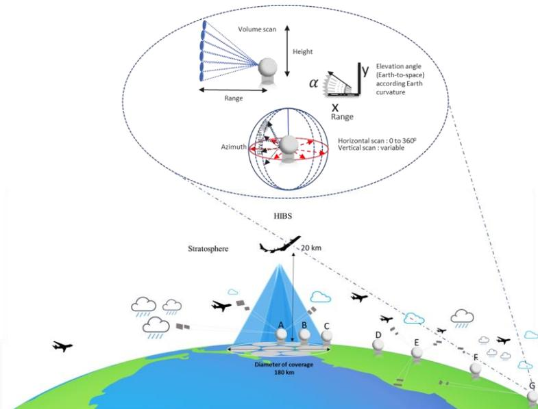
Radar 1: antenna height = 30 m, receiver noise figure = 2.7 dB, horizontal scan:  $-180^{\circ}$  to  $180^{\circ}$ , vertical scan:  $-0.5^{\circ}$  to  $20^{\circ}$
