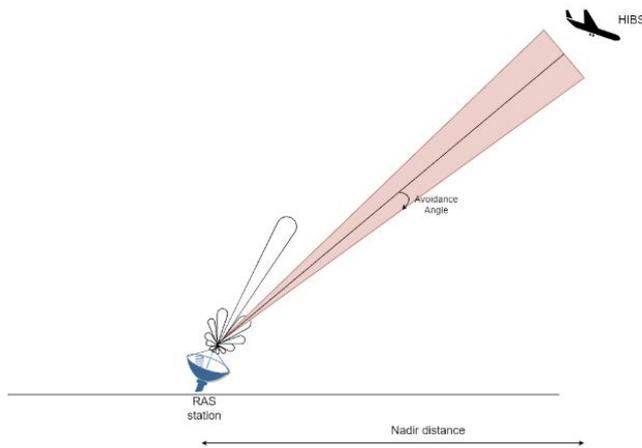
For only one HAPS in line of sight, the maximum permitted sky loss is of 2%, representing an avoidance angle of  $11.5^\circ$ . The gain for an RAS antenna as defined in Rec. ITU-R SA.509, irrespective of antenna diameter, for this off-axis angle is 5.5 dBi.
