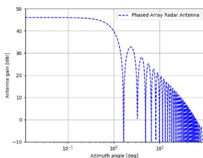
(a) Azimuth antenna pattern
