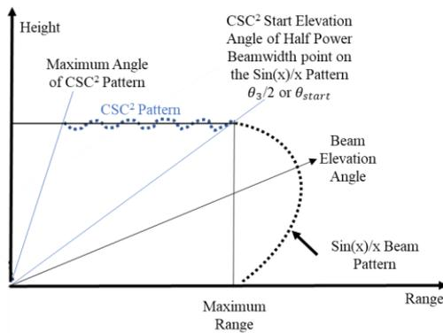
An example using the above procedure provides an antenna pattern for radar B and shown below.
