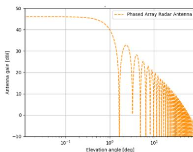
(b) Elevation antenna pattern
