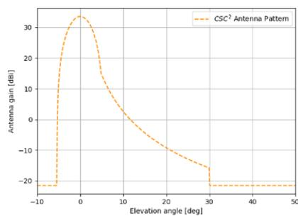
(b) Elevation antenna pattern
