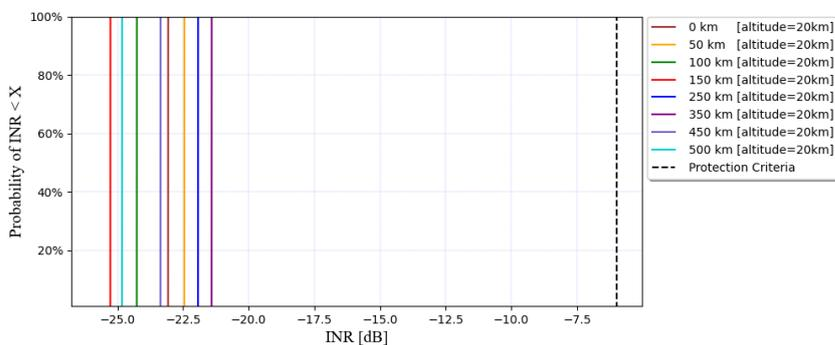
Additionally, the simulations for adjacent channel compatibility analysis were done considering HIBS central frequency at 2 017.5 MHz, and FS (PP) central frequency at 2 032 MHz, as shown in Figure A3.6.1.8.
