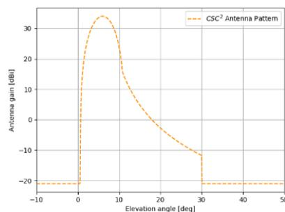
(b) Elevation antenna pattern
