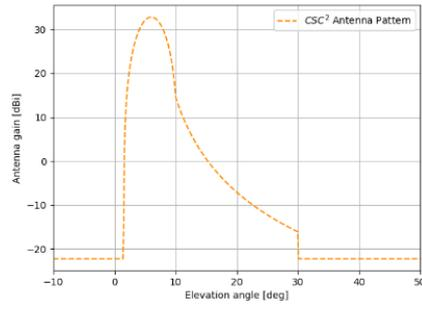
(b) Elevation antenna pattern
