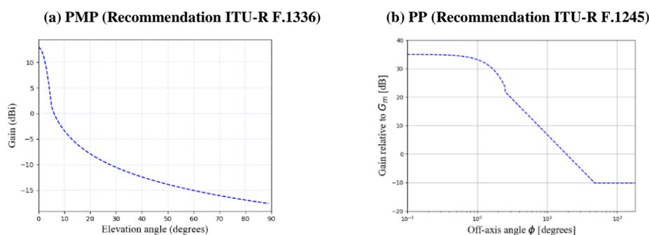
For FS (PP), it should be highlighted that in cases of analysis consisting of many interference entries, as with the HIBS multiple cells, using a peak envelope radiation pattern would result in aggregate interference values that are greater than values that would be experienced in practice. In this case, it is more appropriate to use an antenna pattern in accordance with Recommendation ITU-R F.1245, representing average sidelobe levels.
