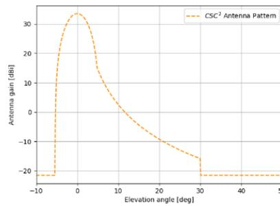
(b) Elevation antenna pattern
