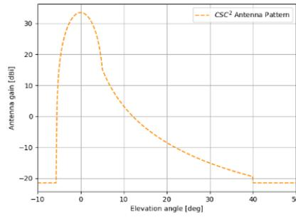
(b) Elevation antenna pattern
