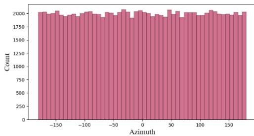
(b) Uniform distribution of azimuth scan
