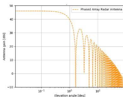
(b) Elevation antenna pattern
