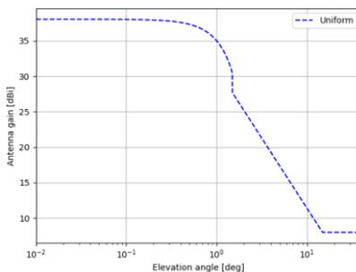
**(b) Elevation antenna pattern**
