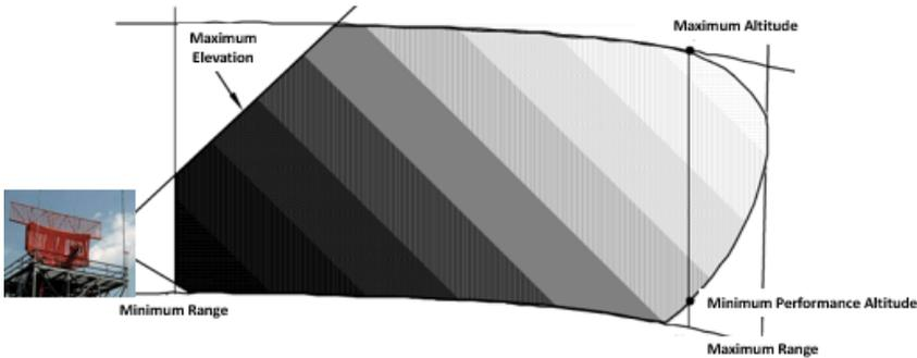
These radars operate using two beams, a low beam, and a high beam, with offset from each other in elevation as portrayed below. In this study the low and high beams susceptibility to possible interference from a HIBS platform located at a maximum height of 20 km was evaluated. The analysis is not valid for other HIBS altitudes. Typical antenna patterns for both high and low beams are shown in the figure below.
