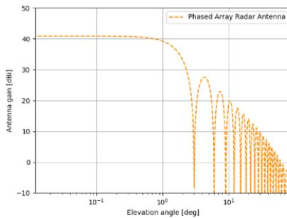
**(b) Elevation antenna pattern**
