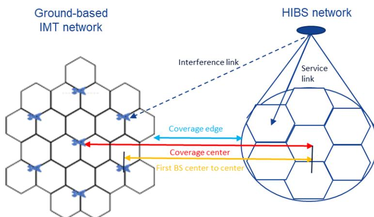
For the evaluation of interference into the ground-based IMT network due to HIBS base station transmissions, this study considers the distance between the coverage centers of the two networks, namely the **Inter-Network Distance (IND)**. Given that the coverage area of the HIBS network has a radius of 90 km and the ground-based IMT cell/sector radius is 0.8 km (inter-site distance 1.2 km) for the assumed suburban environment, one can easily derive the other mentioned distances from the IND.
