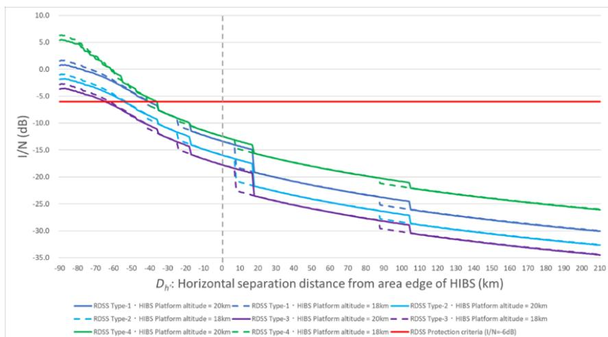
The calculation results of  $I/N$  produced by HIBS at RDSS receiver in Scenario A-2 are shown in Figure A4.5.1.4.
