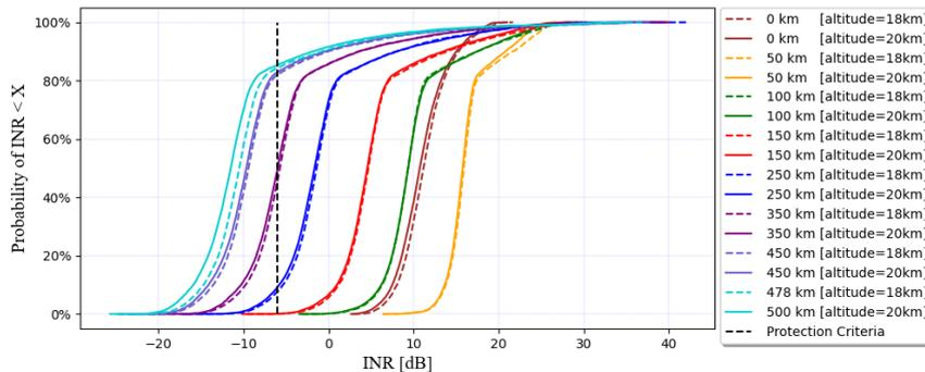
In case no additional measures are implemented for the HIBS station, the results show that the achieved  $I/N$  will not meet the FS (PP) protection criteria of -6 dB. It should be noted that, for this frequency range, Resolution 221 (Rev.WRC-07) currently defines values of power flux-density (pfd) at the Earth's surface for the operation of the HIBS stations in order to protect the FS systems.
