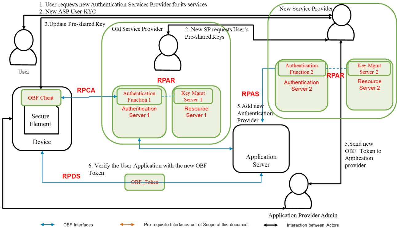
**Figure 10: Change Authentication Service Provider (Symmetric Keys)**
