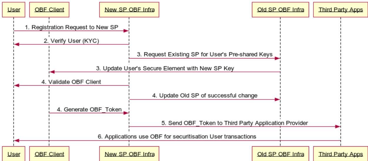
**Figure 110: Change Authentication Service Provider (Symmetric Keys) Sequence**
