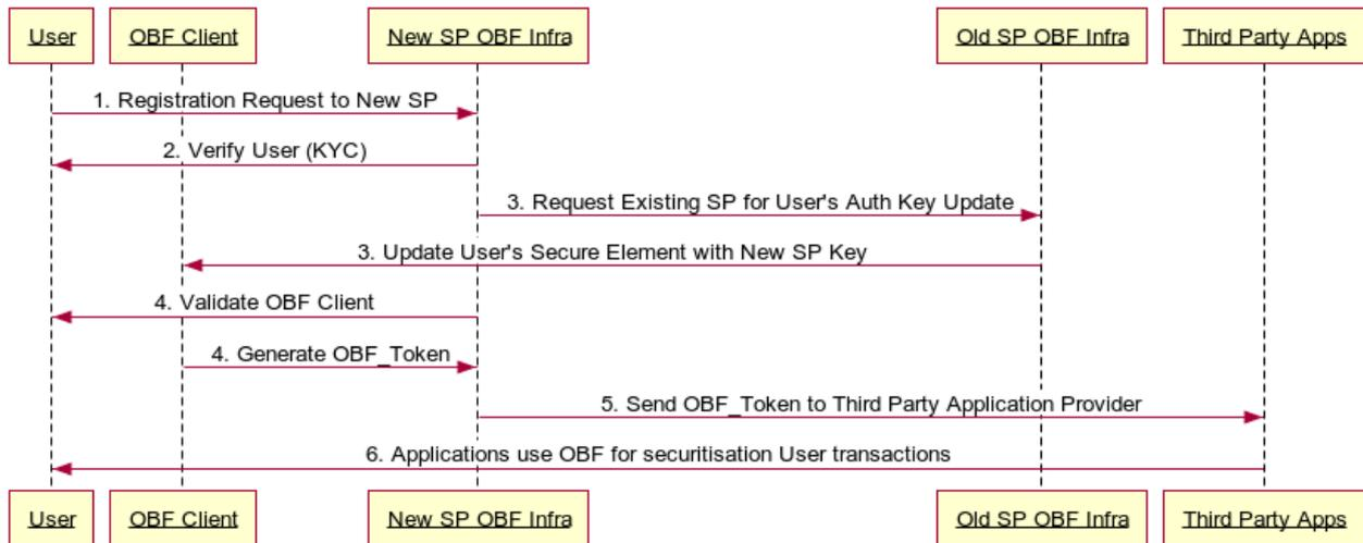
Figure 9: Authentication Provider Switch (Asymmetric keys) Sequence
