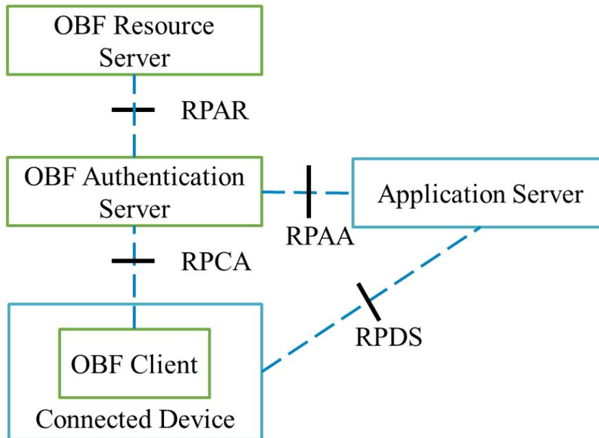
**Figure 2: Functional Architecture showing the OBF Elements**
