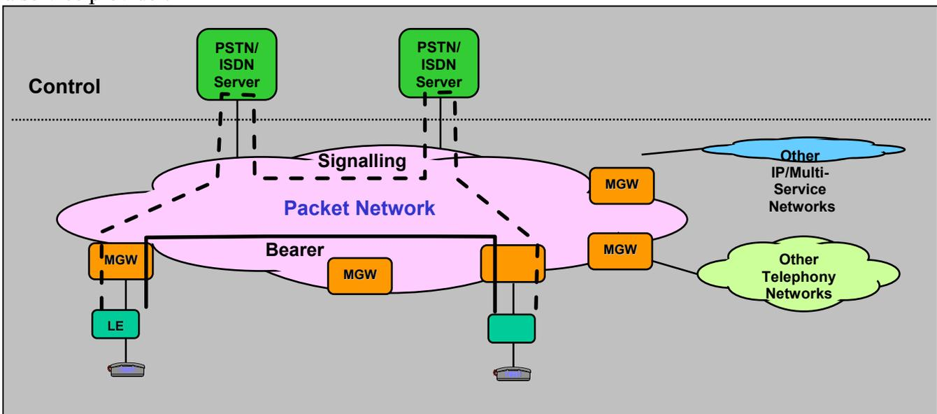
identified by individual packet addresses. The Softswitch sends a BICC request to the nearest Softswitch for determining whether the terminating entity is available in its domain. If it is present then the Packet address of the terminating point on the media gateway is sent back to the originating Softswitch. Once the packet addresses of the terminating end point is determined then control messages are sent to set up the path across the packet network.
