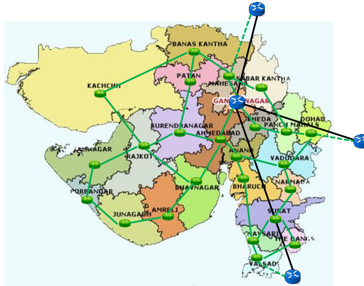
Figure-4: State Broadband Edge Network using MPLS Edge Routers showing connectivity in one State
