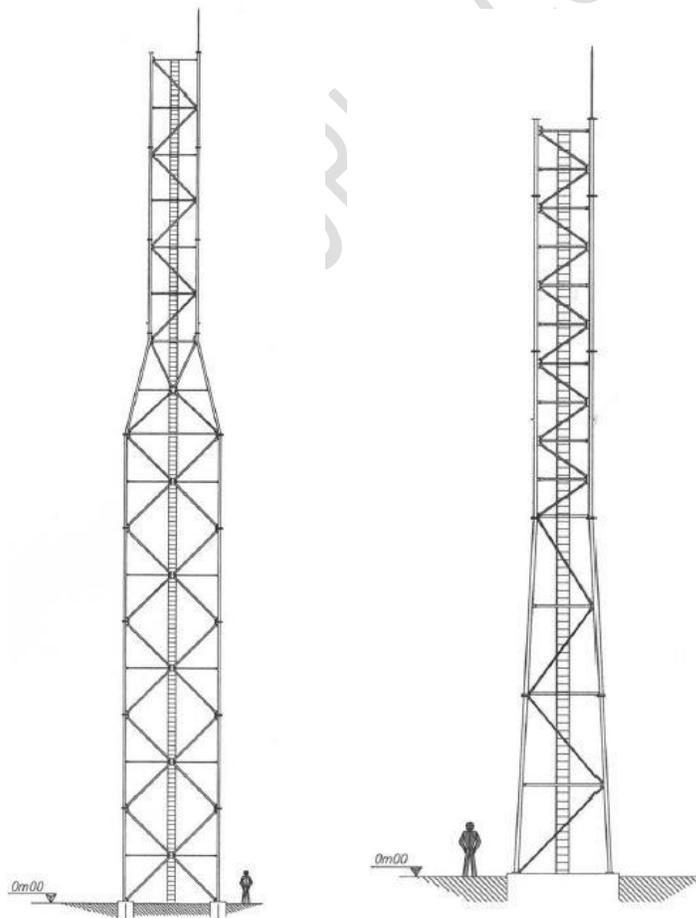
Figure 3: Self-supporting lattice tower
