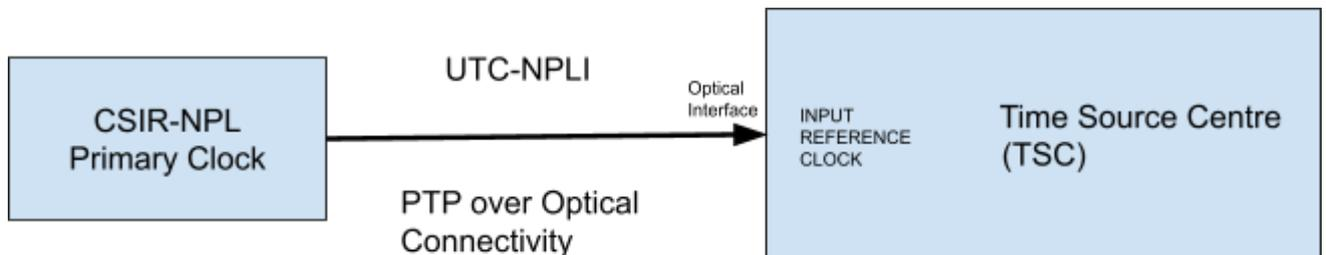
In case of CSIR-NPL Primary Clock Site and TSC are collocated then the input reference to Time Source Centre will be provided by optical connectivity at optical interface. PTP will be provisioned between this optical connection. 1G optical/Electrical interface is required at the PTP GM for input reference from CSIR-NPL
