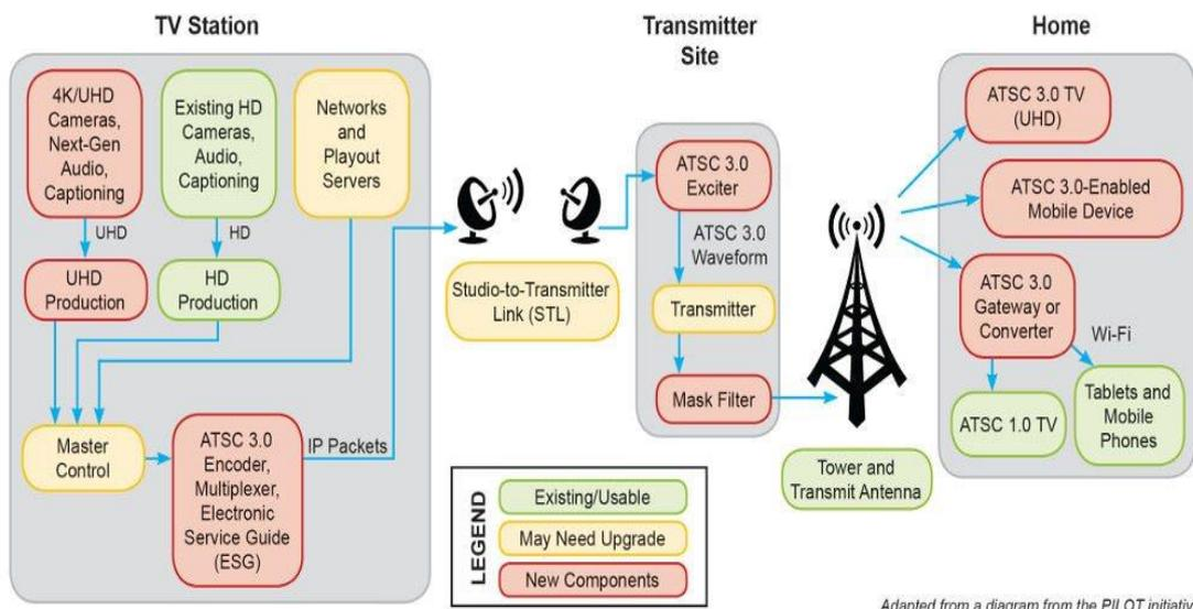
**Figure 6: Block diagram of ATSC3.0**
