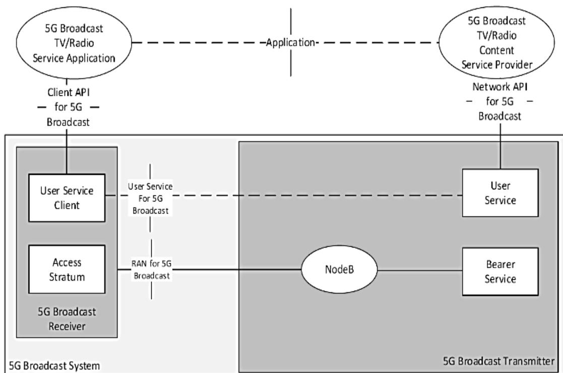
**Figure 5: Reference architecture for 5G Broadcast System**
