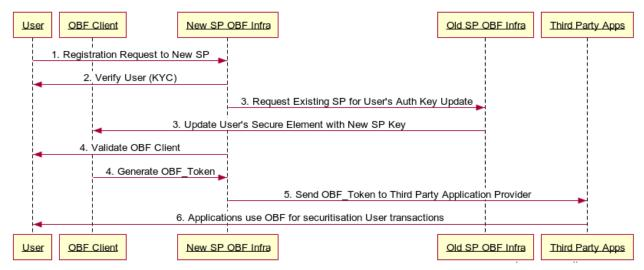
Figure 6: Authentication Provider Change (asymmetric keys)
