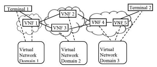
Figure-10 Multi domain end to end virtual network service
