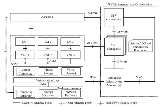
Figure-I NFV high level frame work
