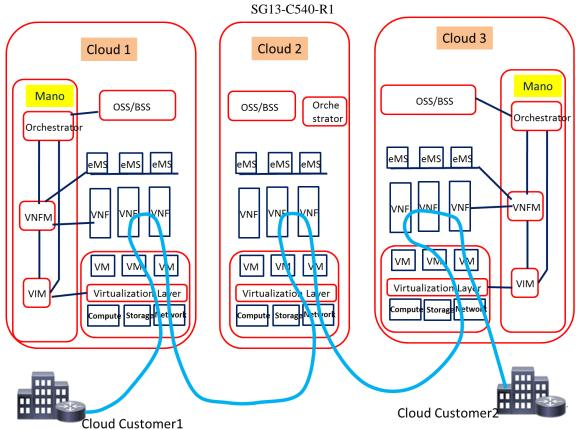
Figure-11 VNF Forwarding Graph for Multi domain end to end service
