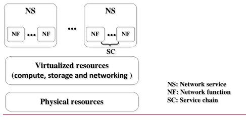
**Figure 6-1 – Virtualization hierarchy of network service**
