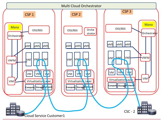
Figure 6-2 – VNF Forwarding Graph for Inter-cloud end to end service
