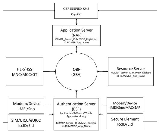
Figure 5. Functional Model of the Open Bootstrap Framework
