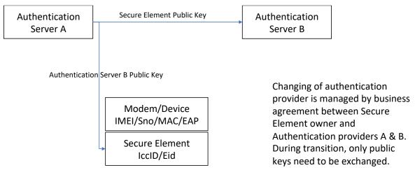
Figure 6. Transfer of Authentication Service Provider
