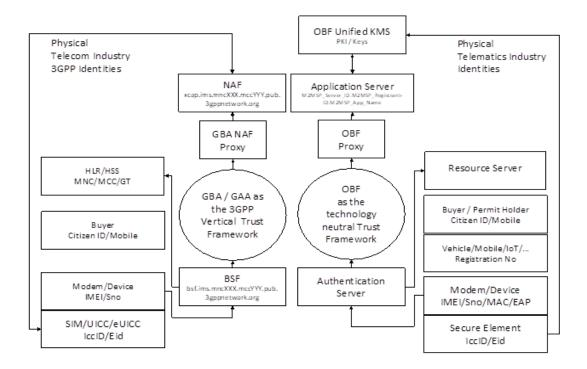
Figure 2. 3GPP and Open Bootstrap Framework Concept
