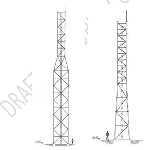
Figure 3: Self-supporting lattice tower
